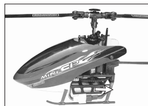
Step 3: Remove the battery pack.
