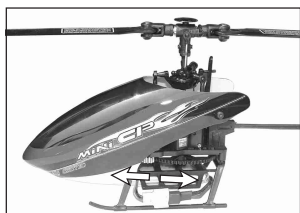
Step 1: disconnect the power cable of helicopter.
